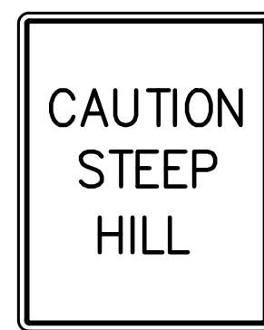
24" x 30" BLACK ON WHITE REFLECTORIZED 7'-0" MOUNTING HEIGHT
